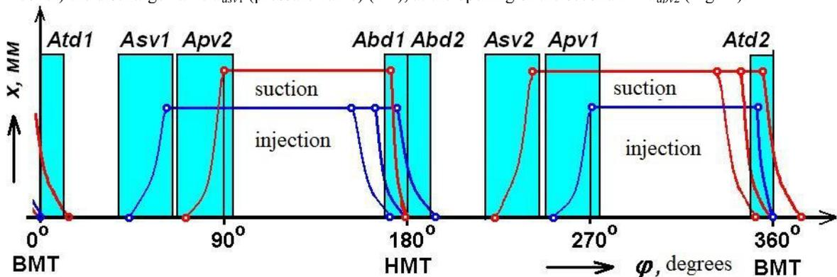
Fig. 1. Cyclogram of working piston compressor (the dependence of the height of the valve plate lift on the angle of shaft rotation).
