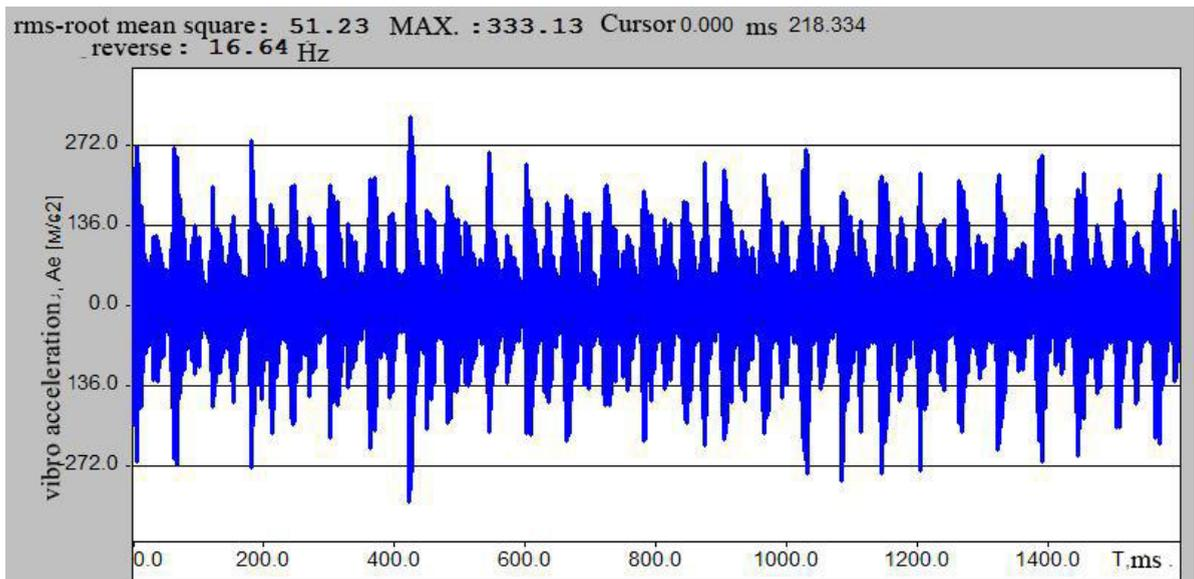
Fig. 4. Signal acceleration  $A_f$  on the cylinder in the axial direction of the piston compressor type JGT/2 Ariel company in the range up to 10 kHz.
