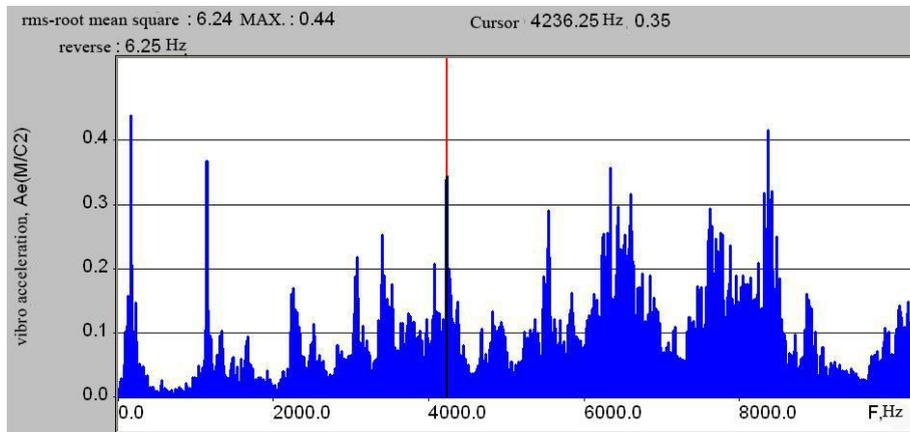
Fig. 3. The range of acceleration  $A_e$  on the cylinder in the axial direction of the piston compressor type 4M16M-45/35-55.
