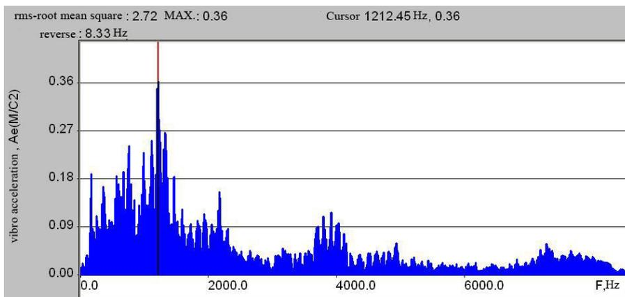
Fig. 2. The range acceleration  $A_e$  on main bearing piston compressor type 2GM16-20/42-60.
