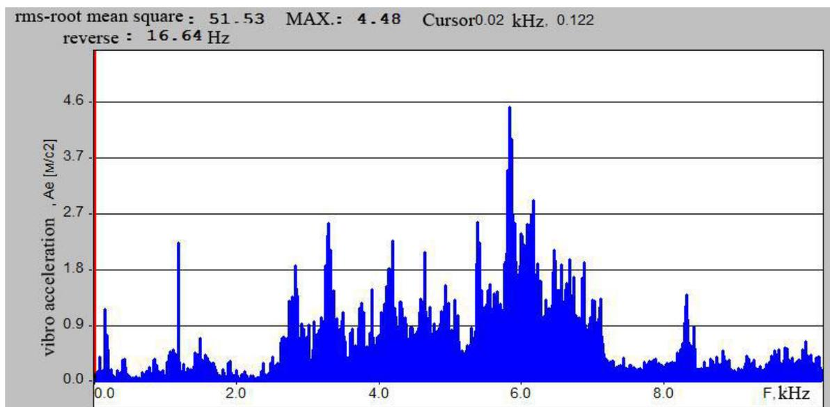
Fig. 5. The range of acceleration  $A_f$  on the cylinder in the axial direction of the piston compressor type JGT/2 Ariel company.
