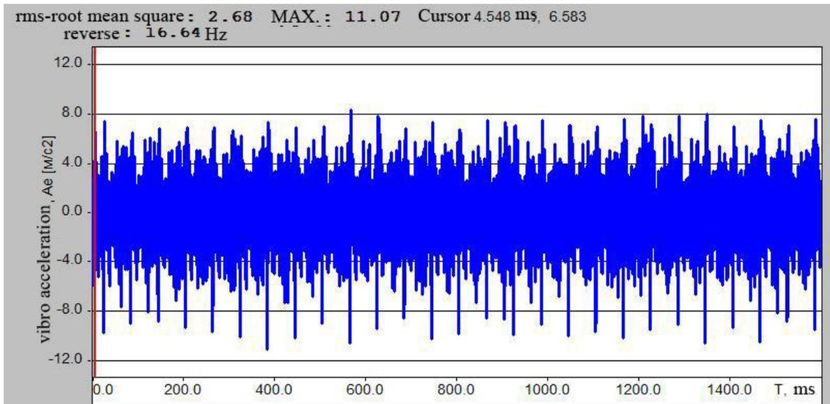
Fig. 6. The signal acceleration  $A_T$  on the cylinder in the axial direction of the piston compressor type JGT/2 Ariel company in the range up to 1 kHz.
