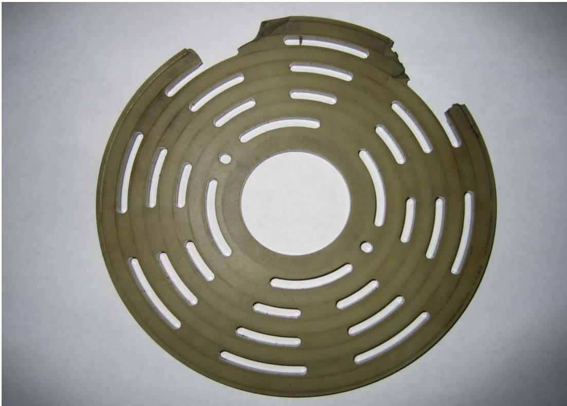
**Figure 4. Destroyed valve plate of the piston compressor**
