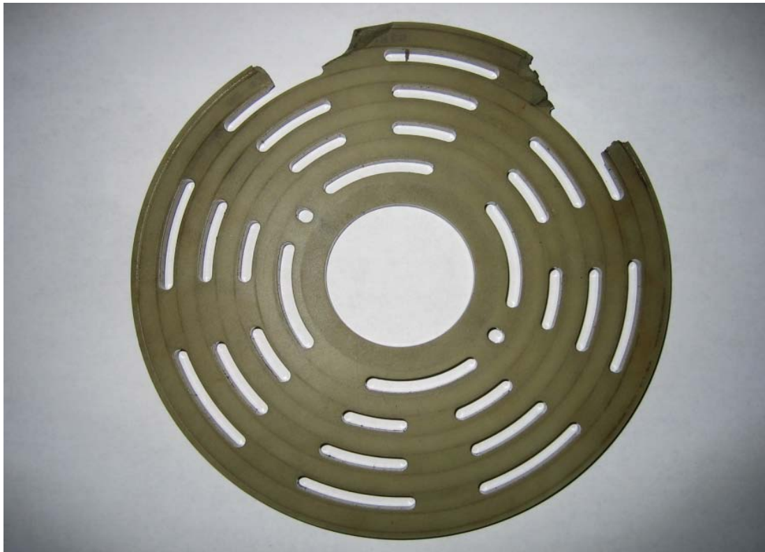
Figure 4. Destroyed valve plate of the piston compressor
